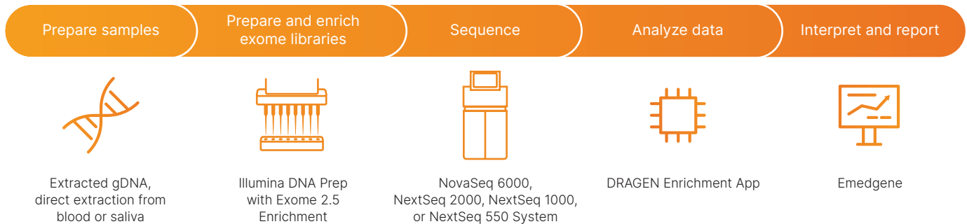
Figure 1: From samples to reporting from a single partner—Illumina supports an end-to-end workflow for WES. Extracted gDNA (or DNA from blood or saliva following direct extraction protocols) is input to library prep with Illumina DNA Prep with Exome 2.5 Enrichment. Qualified Methods are available on a range of automation platforms. Sequence according to scale and throughput needs on Illumina instruments. Accurate, rapid secondary analysis and variant calling is performed with the DRAGEN Enrichment App. For genetic diseases, Emedgene enables intuitive interpretation and reporting.
