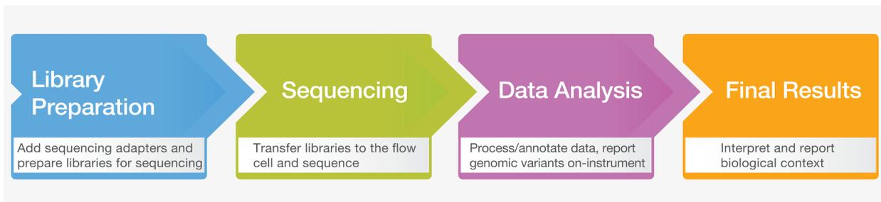
**Figure 2: MiSeq Workflow**—The streamlined workflow of the MiSeq System enables rapid turnaround time for next-generation benchtop sequencing. Libraries can be prepared with any Nextera library preparation kit. Five and a half hour sequence time includes cluster generation, sequencing, and quality-scored base calling with dual surface scanning for a 2 × 25 base pair run on a MiSeq System with MiSeq Control Software.
