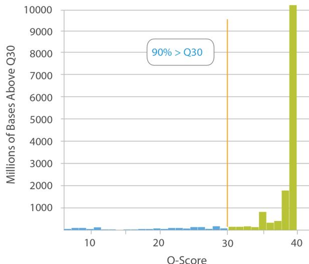
**Figure 3: MiSeq quality score distribution**—Quality scores for a PhiX control library, 2 × 300 base pair run on a MiSeq System with MiSeq Control Software v2.4. This example shows 90% of bases sequenced above Q30.
