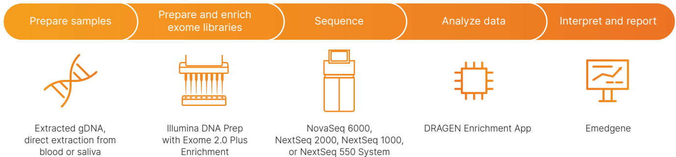
Figure 1: From samples to reporting from a single partner—Illumina supports an end-to-end workflow for WES. Extracted gDNA (or DNA from blood or saliva following direct extraction protocols) is input to library prep with Illumina DNA Prep with Exome 2.0 Plus Enrichment. Qualified Methods are available on a range of automation platforms. Sequence according to scale and throughput needs on Illumina instruments. Accurate, rapid secondary analysis and variant calling is performed with the DRAGEN Enrichment App. For genetic diseases, Emedgene enables intuitive interpretation and reporting.
